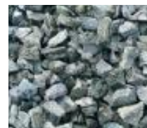
CGA Type 4/20 (clean stone) - permeable
