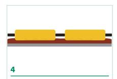
Once the formation has been agreed, measure and cut the Flexible Pipe to join the tanks together use 2x O-rings per connection to create a strong seal.
