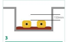
Position the tank within the planting area ensuring the capillary leg top is a maximum of 150mm from the lowest roots of the plant(s). Ensure the links are no more than 400mm apart.
