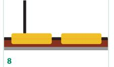
Install the Filler Pipes into the Mona links. Pipes are pre-assembled and may require cutting - it should be flush with the finished surface level. Ensure there is a filler pipe every fifth Mona link.
